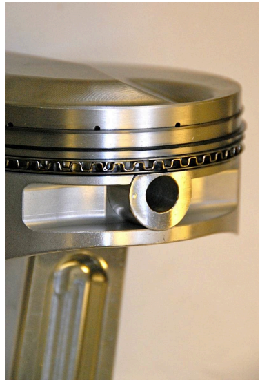
Zoom on grooves and the drain system for oil from www.engine1abs.com
