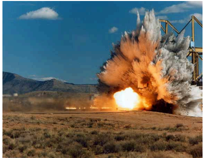
Crash test of supersonic jet fighter McDonnell Douglas F-4 against a reinforced concrete target Sandia National Lab
