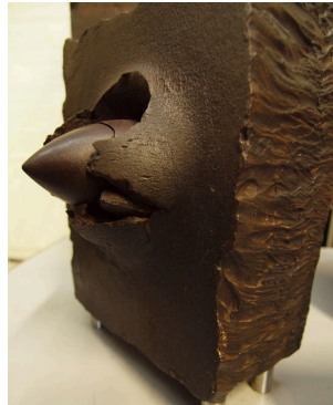
Sherman Firefly armor piercing shell on Tiger tank armor, Bovington Tank Museum Andy's photo www.flickr.com
