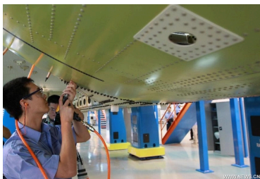
Fuselage of modern aircraft contains \approx 100\,000 rivets www.news.cn
