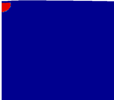
Evolution of the plastic zone in a sinusoidal asperity in contact with a rigid flat
