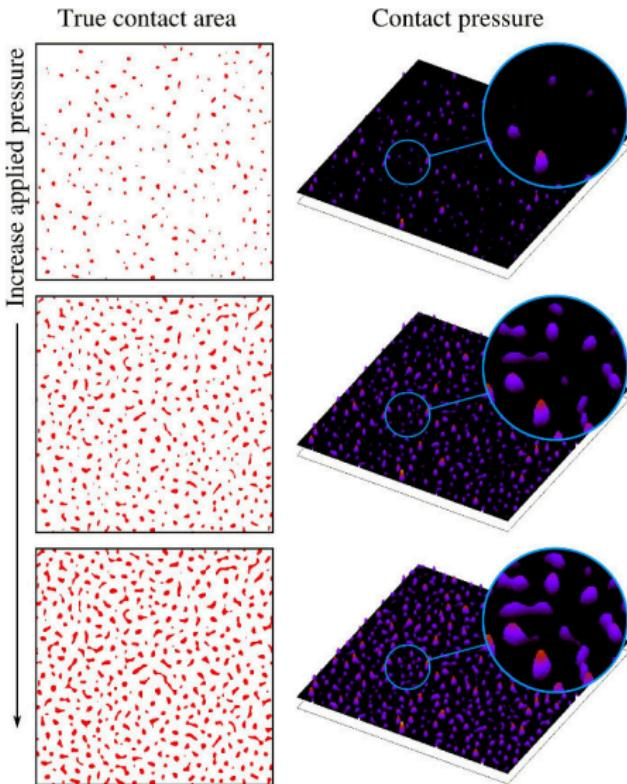
Fig. True contact area and stress fluctuations
