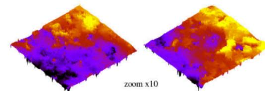
Fatigue & creep fracture surfaces (Ti-alloy)
