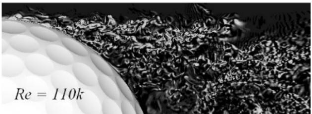
Fig. Numerical simulation of airflow around a (dimpled) golf ball [5]
