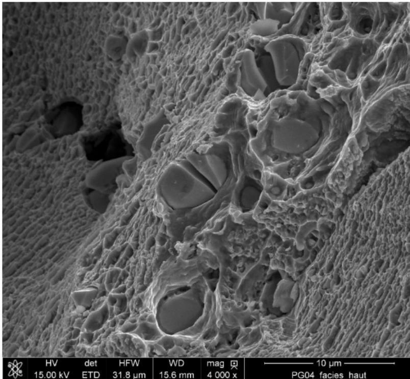
Fatigue fracture surface (Co-alloy), particles WC
