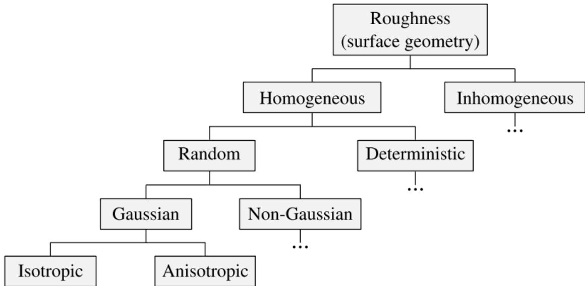
Fig. Roughness classification according to Nayak<sup>[1]</sup>
