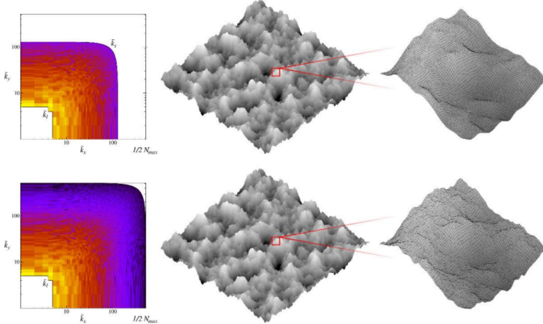
Fig. Power spectral densities (Fourier space) and corresponding rough surfaces (real space) for
