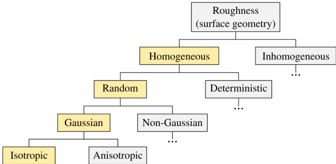
Fig. Roughness classification according to Nayak<sup>[1]</sup>
