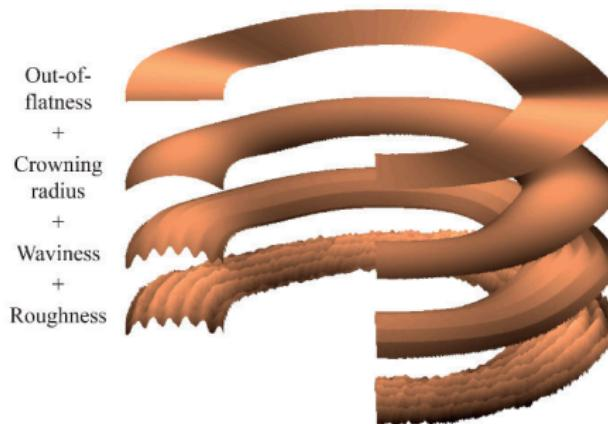
Fig. Circular metallic seal with turned copper surface<sup>[1]</sup>
